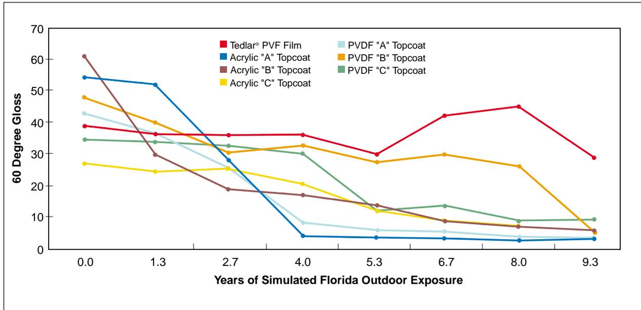
The Tedlar® PVF film shows excellent gloss retention after the equivalent of nearly 10 years of exposure, while the coating materials have failed to maintain their integrity. In fact, because the protective layers of the coating materials have been essentially depleted, both color and gloss measurements on these systems are probably the properties of the PVC substrate alone.
