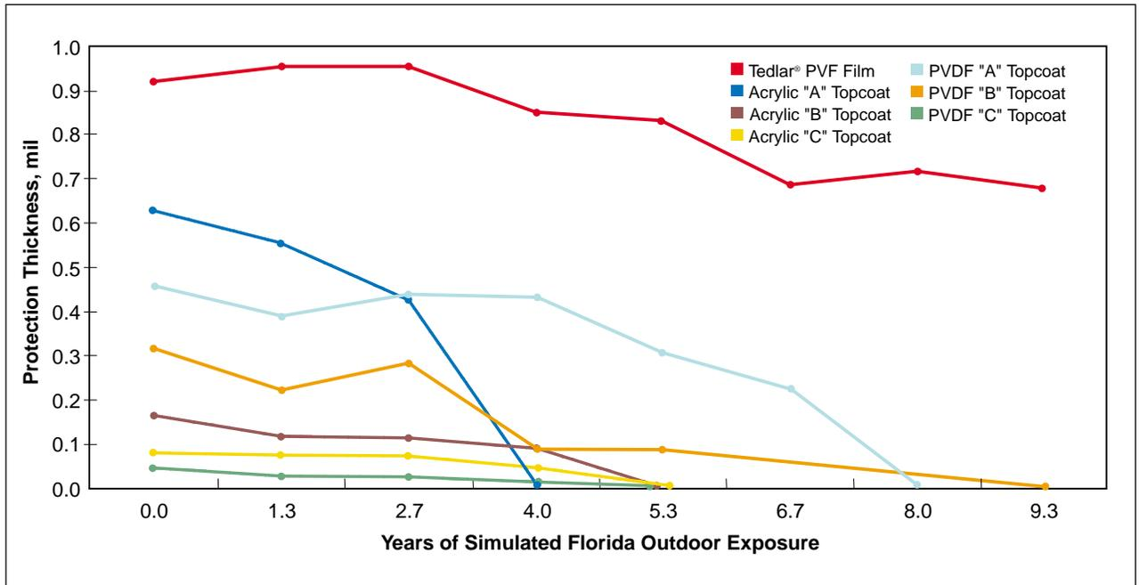
**Note:** This simulation shows that Tedlar® protective film not only starts out thicker than any of the other protective coatings, but retains superior thickness long after the others eroded completely.
