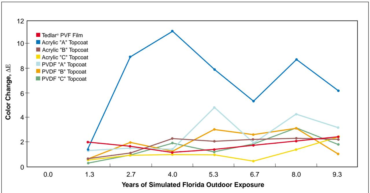
Color change can be attributed to degradation by UV light and dirt pickup. Note that the Tedlar® PVF film shows no color change after the equivalent of nearly 10 years of exposure.
